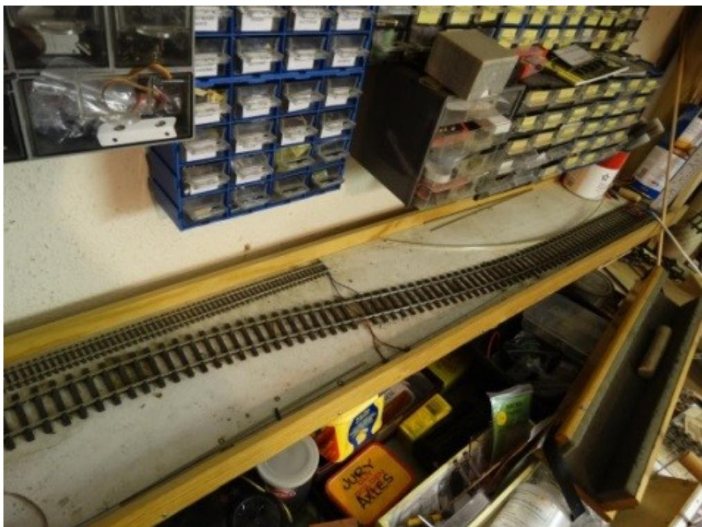
It usually becomes a shelf in the workshop but has been specially cleared for the photo. In addition to its basic shape the track can be pushed to tighten the curve beyond the nominal radius, in this case 4 feet\*; and to check the flexibility of a chassis the rails can be lifted; illustrated here by wedging a screw driver under the track. Both inside and outside of the curves can be lifted.
