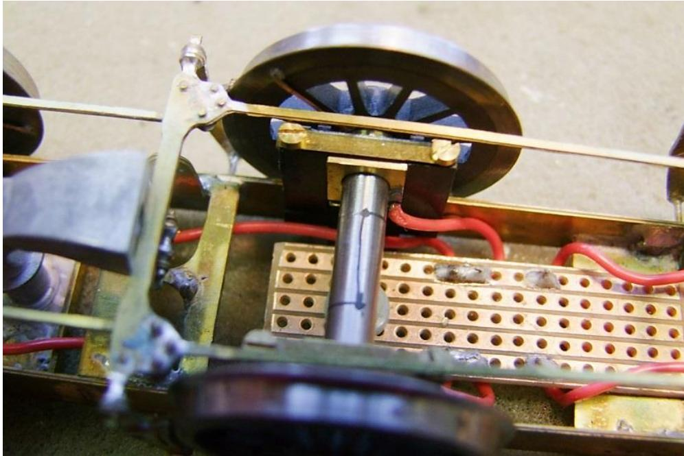
A wire is soldered to the bearing and, in the example shown, taken to piece of Veroboard from which two wires go forward to the motor.
