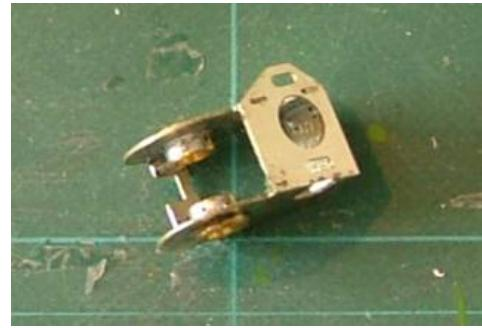
Solder the bushes to the sides with the jury axle in place. The axle should rotate freely after soldering showing that both bores are in line. This is unlikely to happen if the bushes are fitted at an earlier stage.
