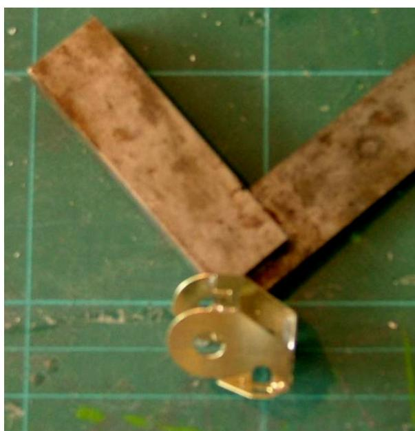
The second side was added and the closure across the two side plates soldered in place. All the fold lines have a generous fillet of solder to reinforce them. Check after doing this that the corners remain square as the solder can pull them in.
