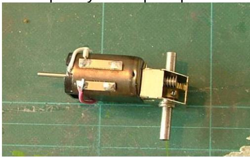
Run the motor in each direction without any load on the jury axle. There should be minimal noise from the mesh and at full speed the motor whine should be louder. Repeat using fingers to apply a braking load to the jury axle. Again there should be little noise from the mesh. If it noisy then the mesh is too slack and the worm engaged a little deeper with the gear. Try again.
