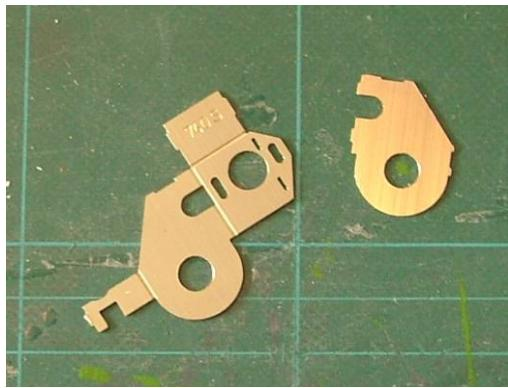
The instructions for this unit quote that the axle bearings should be fitted to the sides before assembly. I would disagree with this and in every case will fit the bearings to the assembled gearbox etch.
