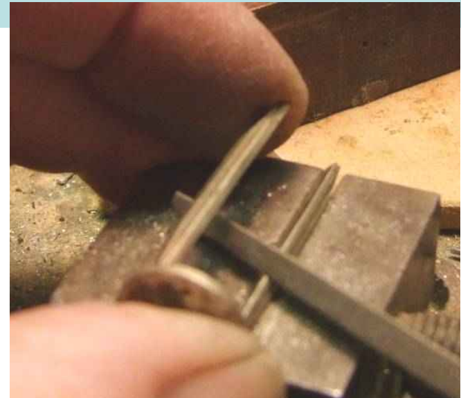
Use a triangular file to clean-up the slidebars. It's stiffer than a flat file so it will not round the running surfaces
