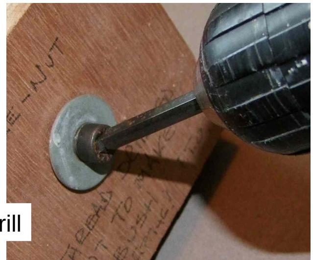
I standardise on M6 Allan headed machine screws for **all** joints
