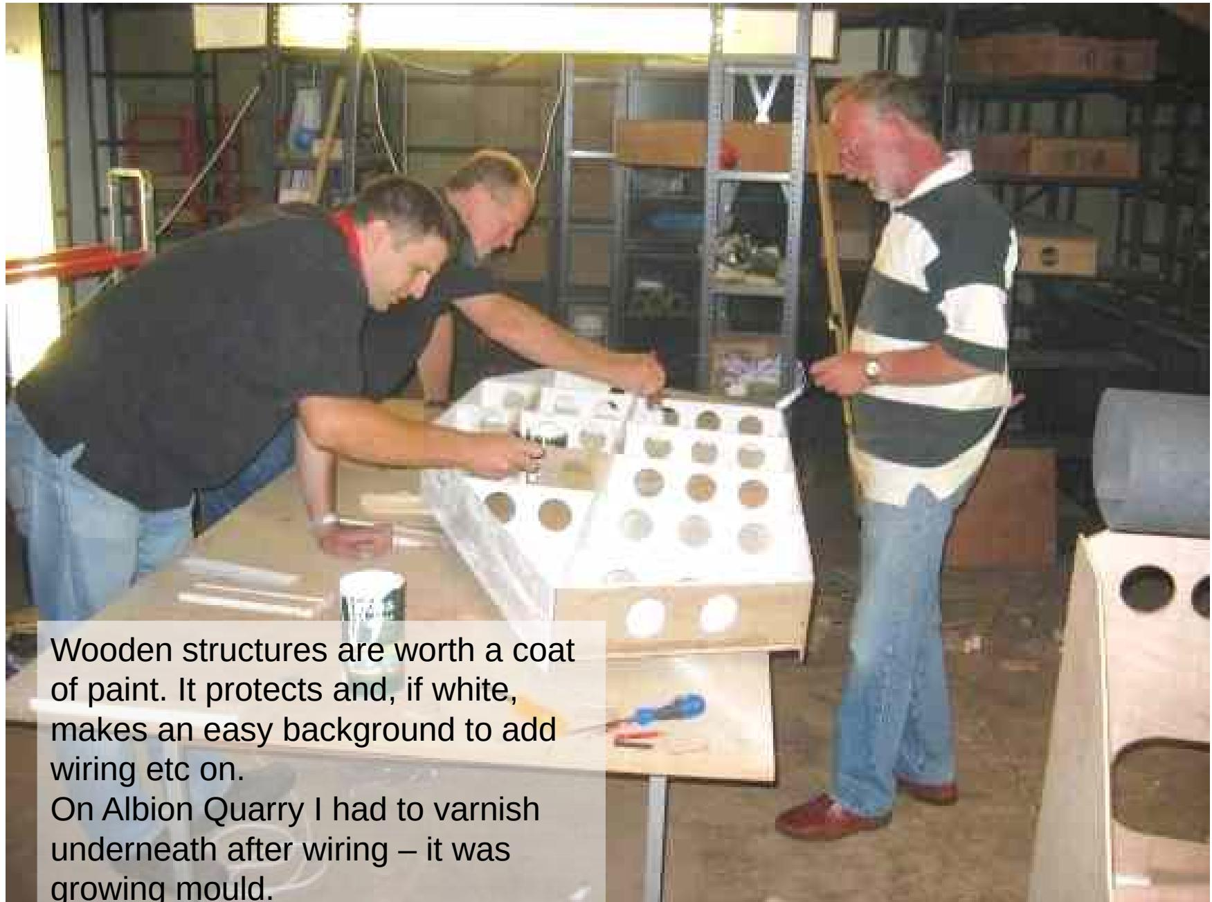
Wooden structures are worth a coat of paint. It protects and, if white, makes an easy background to add wiring etc on.
