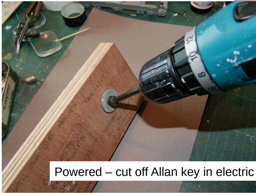
Powered – cut off Allan key in electric drill
