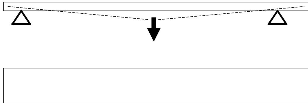
The deeper the section the stiffer they will be. This also makes more room for point motors etc.
