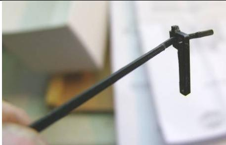
Clean up the brake handles to remove mould marks and assemble over the handle guides before fitting them to the chassis. Use no adhesive at this stage.
