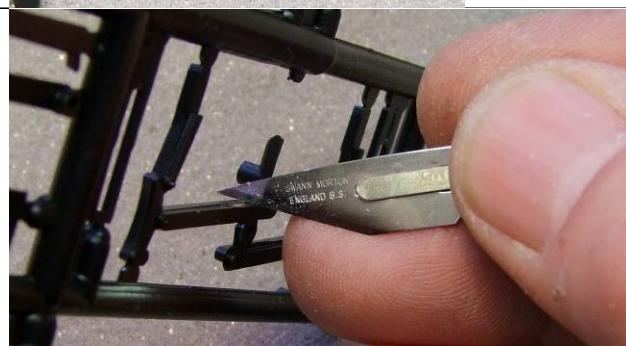
Some parts are best trimmed whilst still attached to the sprue. Typically here there is a register of the mould halves. This is scraped away with a scalpel blade.
