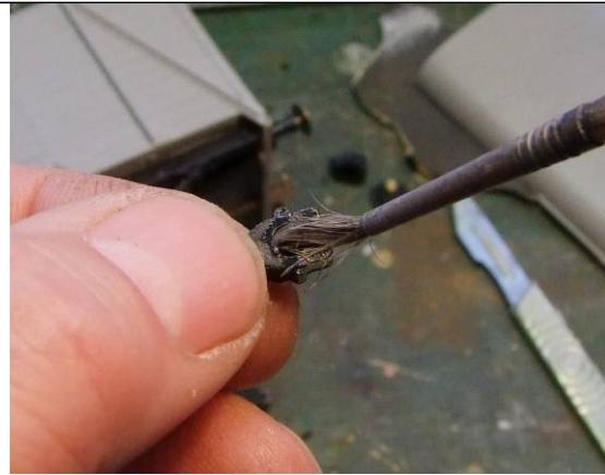
The axleboxes are then glued onto the inner bearings. Apply the adhesive into the hole. Do not have it swimming in adhesive. Fit the axlebox over the brass bearing. To stop the axlebox adhering to the W iron a light application of saliva to the surface will prevent this.
