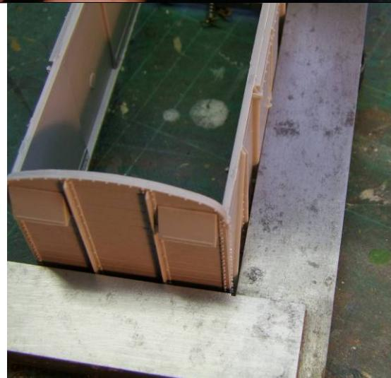
The typical construction of plastic wagons with bevelled joint at each corner means that it possible to assemble the ends and sides without the floor. Assemble one end and one side to form an "L" shape aligning the corner. Repeat for the other two. Join these two assemblies and check they are square. The joints will be flexible initially so can be pushed around. The large square being used to check that everything is at right angles
