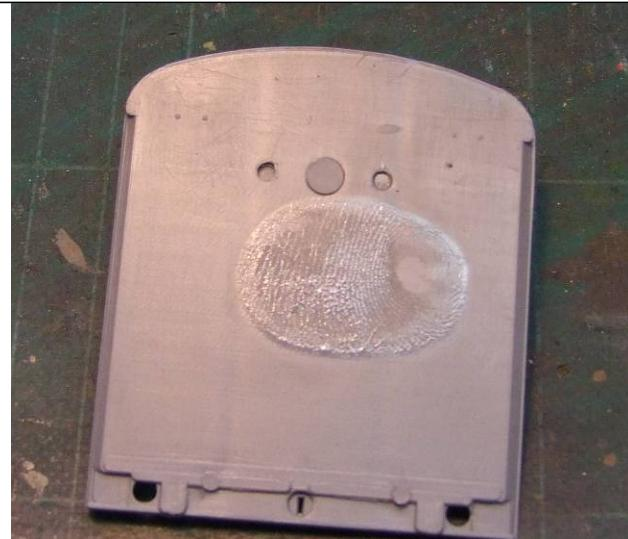
However a misplaced thumb whilst the adhesive is still wet results in a permanent impression. Disaster on a detail surface.
