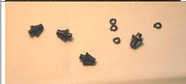
The buffer bodies and the ring that completes their shape have been trimmed from the sprue. Note the rings need further trimming.
