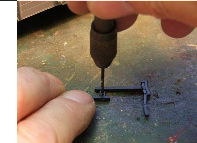
Other brake gear parts required drilling.
