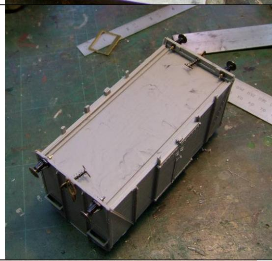
Once the ends and sides are secure the floor can be trimmed and fitted. In this instance the floor locates the solebars in grooves. Material has to be removed equally from each side to maintain symmetry. The floor can then be fitted from above to sit on its locations on the ends and between the sides.
