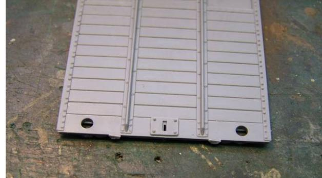
The part removed from the sprue. Note that there are still large registers of its attachment. This is deliberate as it much easier to trim them exactly when they accessible without the sprue.
