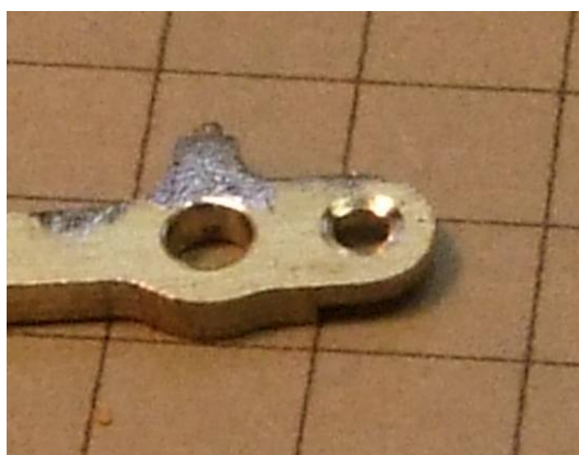
The edge of the hole should look something like this after countersinking.
