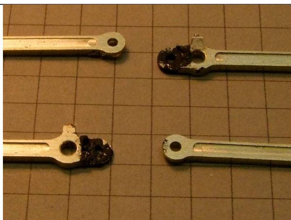
Coat the inside face of the joint with Carr's Solder Mask
