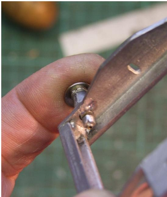
The sole bars were then drilled for the tie down rings.
