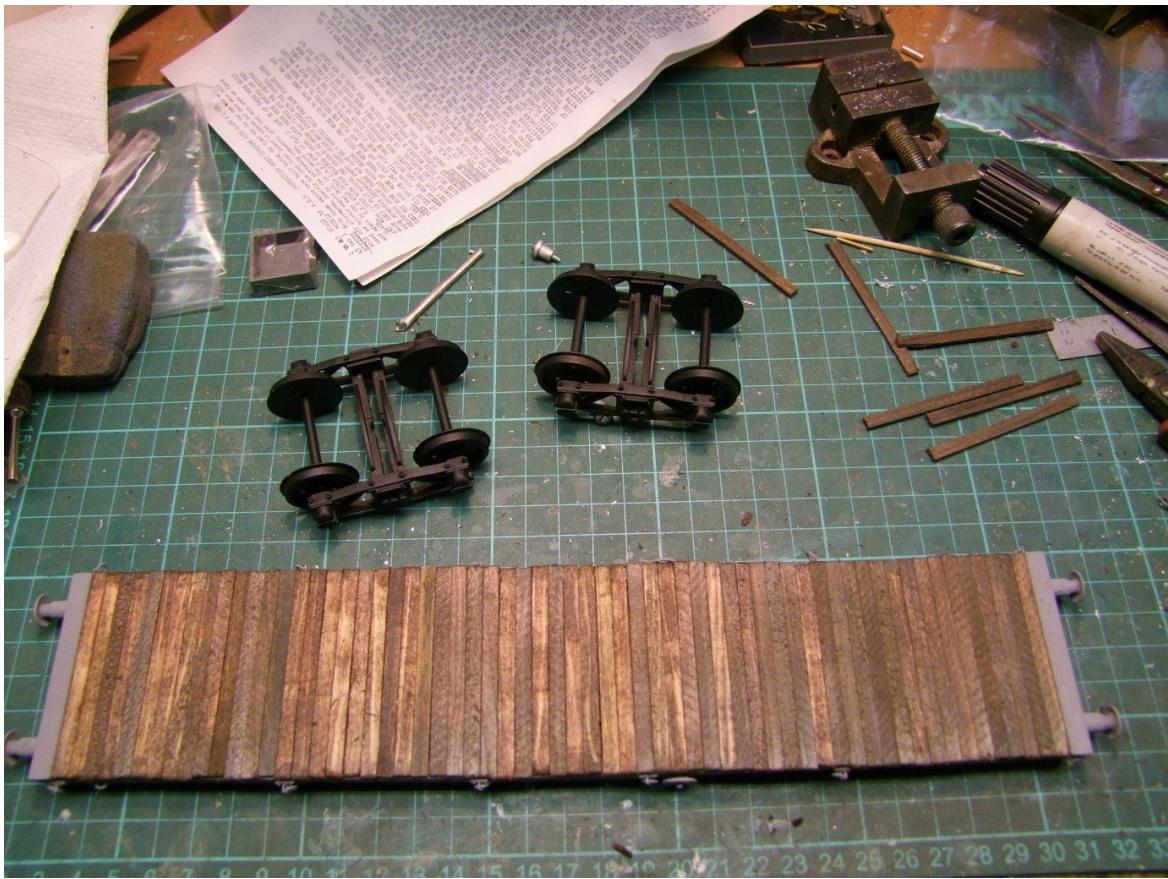
I brush painted the underframe with Railmatch acrylic LNER Wagon grey and applied HMRS Pressfix transfers from their LNER wagon sheet. The correct lettering has to be derived from other wagon names on the sheet.
