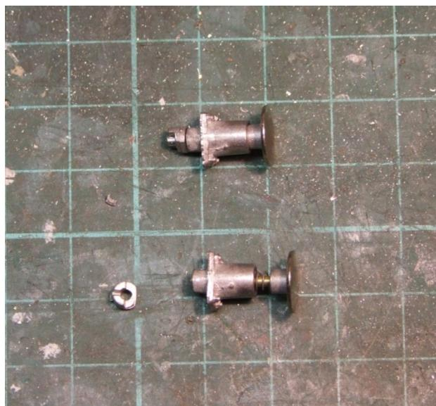
The buffers were inserted into the headstock and soldered from behind.
