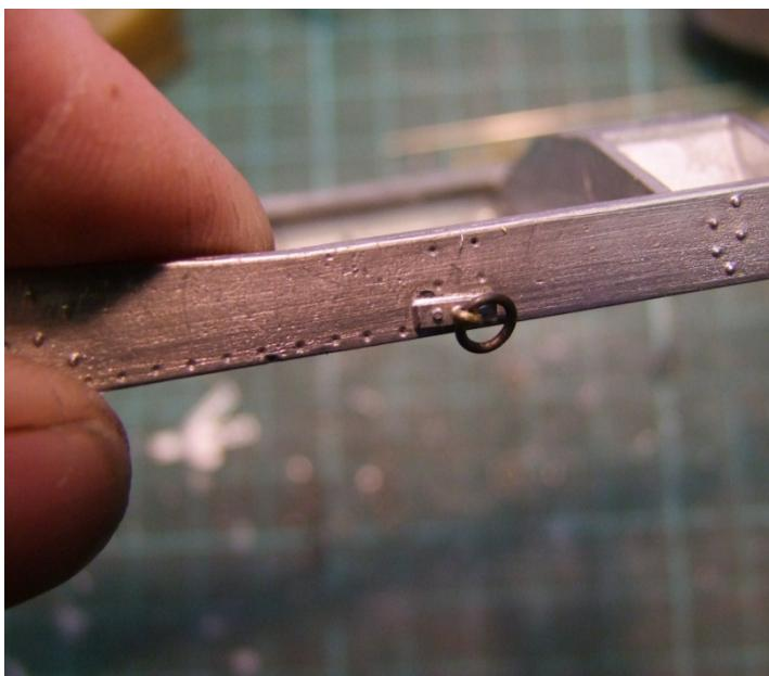
Rather than using the whitemetal rings supplied I made new ones from brass wire. This was annealed and wound around the shank of a drill
