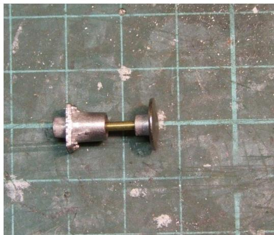
The spring is compressed and the stop soldered to the tube. This is much, much easier than you think.
