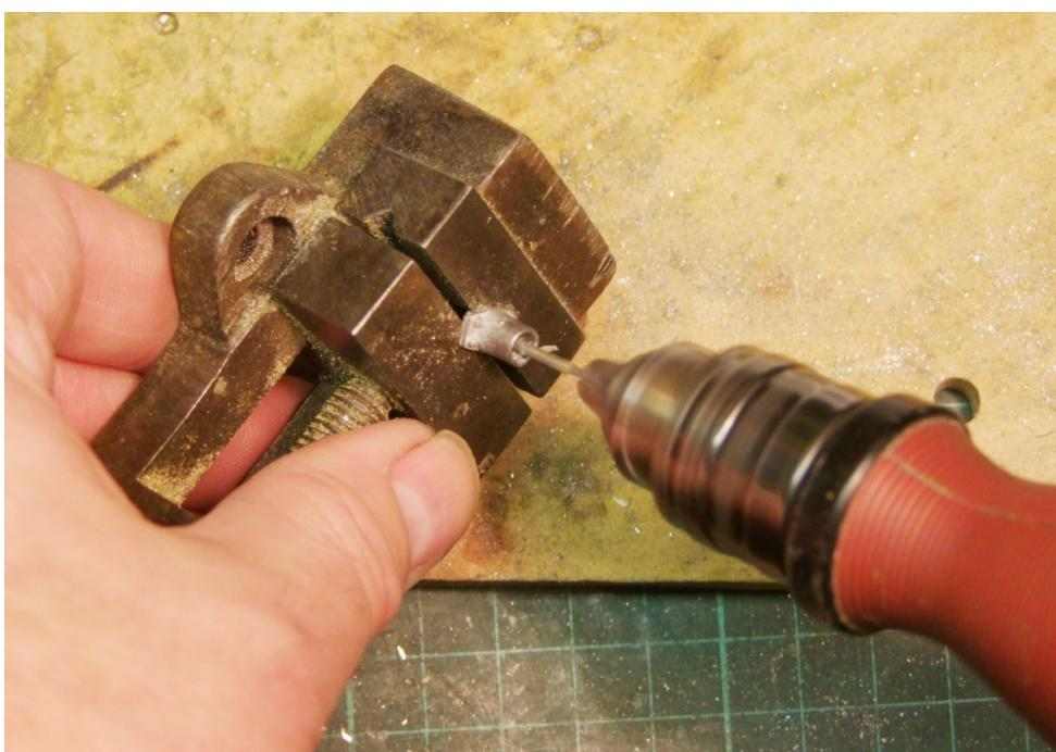
The buffers are a novel assembly of a drawing pin, a brass tube and whitemetal parts. The tube has to be cut to length. The easiest way to cut the tube is to roll it under a Stanley knife blade to create a groove. The tube can be snapped on the groove. The raised burr needs to be filed off.
