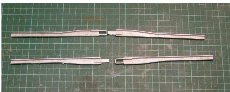
Both parts need some cleaning up so they join cleanly. Material was removed from the outside of the tab and the inside of the "slot".
