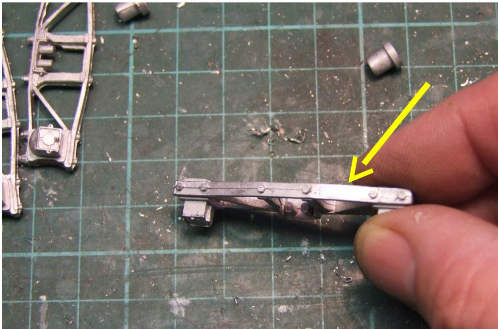
Once cleaned up the bogie sides need drilling for the brass wheel bearings. The first hole was cautiously drilled until the required depth was found. The drill was then marked so that when drilling the remaining holes there was indication of when to stop.
