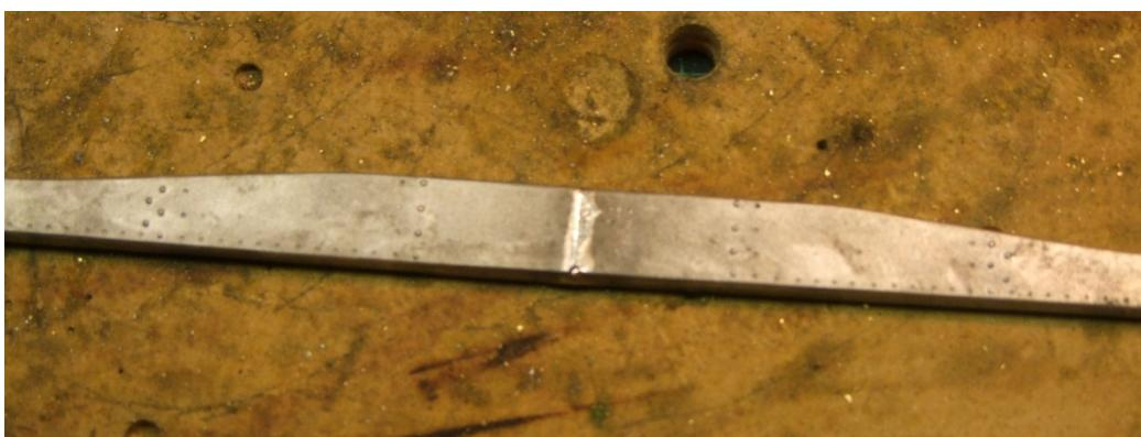
The Carr's 100° solder has good fluidity and fills gaps well. Similarly it flows well around the internal parts of the joint. The solder is taken to the joint on the tip of the iron just as for soldering brass and nickel silver.
