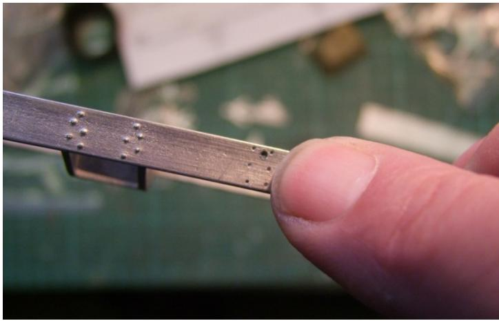
The fixing plates and split pins were soldered in place from behind. The solder is fluid enough to run through the hole and under the plate.
