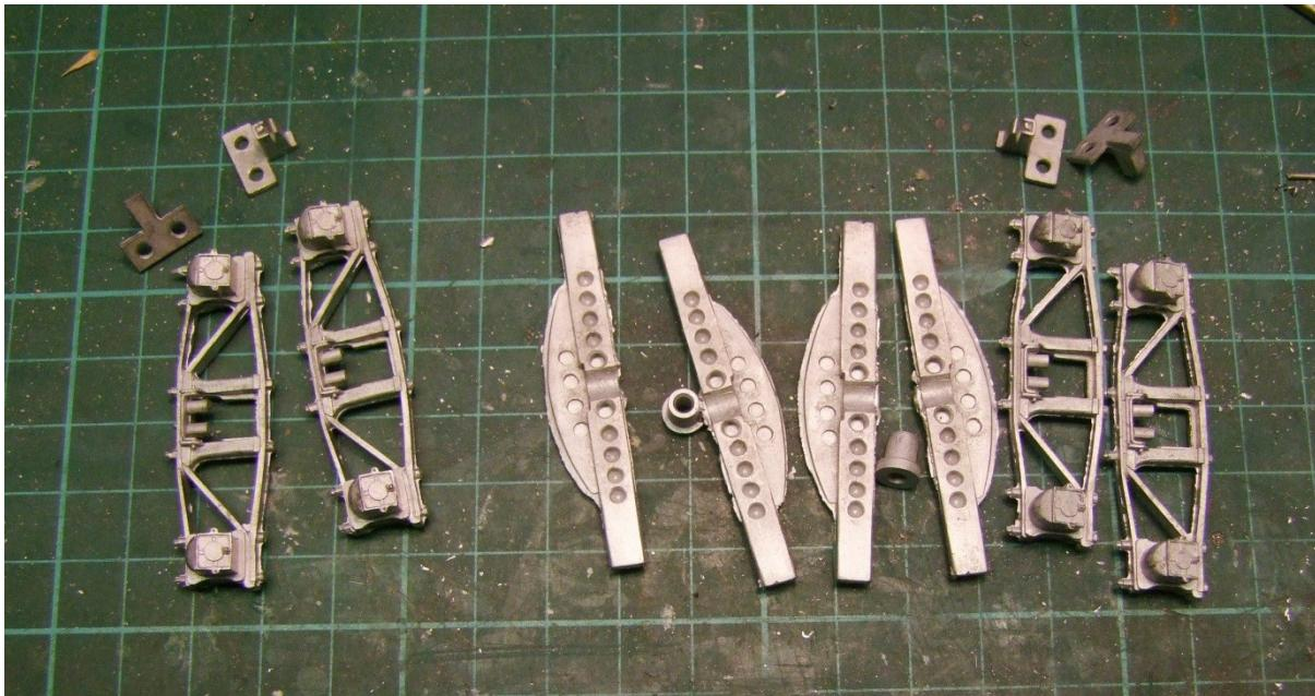
Once again the parts required some cleaning up. Paring off flash with a scalpel or scraping off a mould line.
