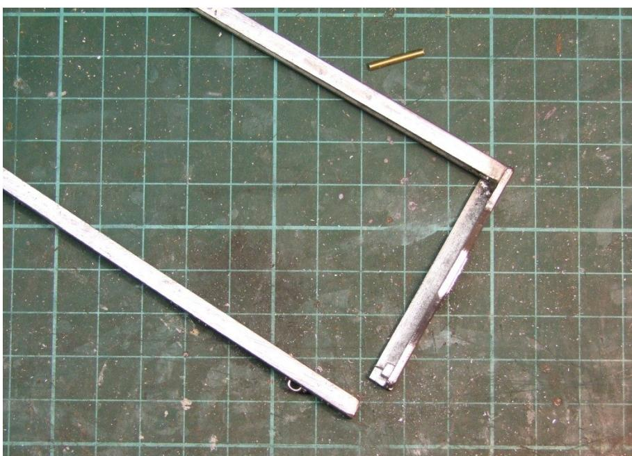
The "L" shapes were then joined to make a rectangle of the underframe.
